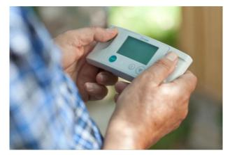
Figure 1. The Zenicor EKG-2 device used to acquire single-lead, 30-second ECG recordings in the SAFER Feasibility Study.
