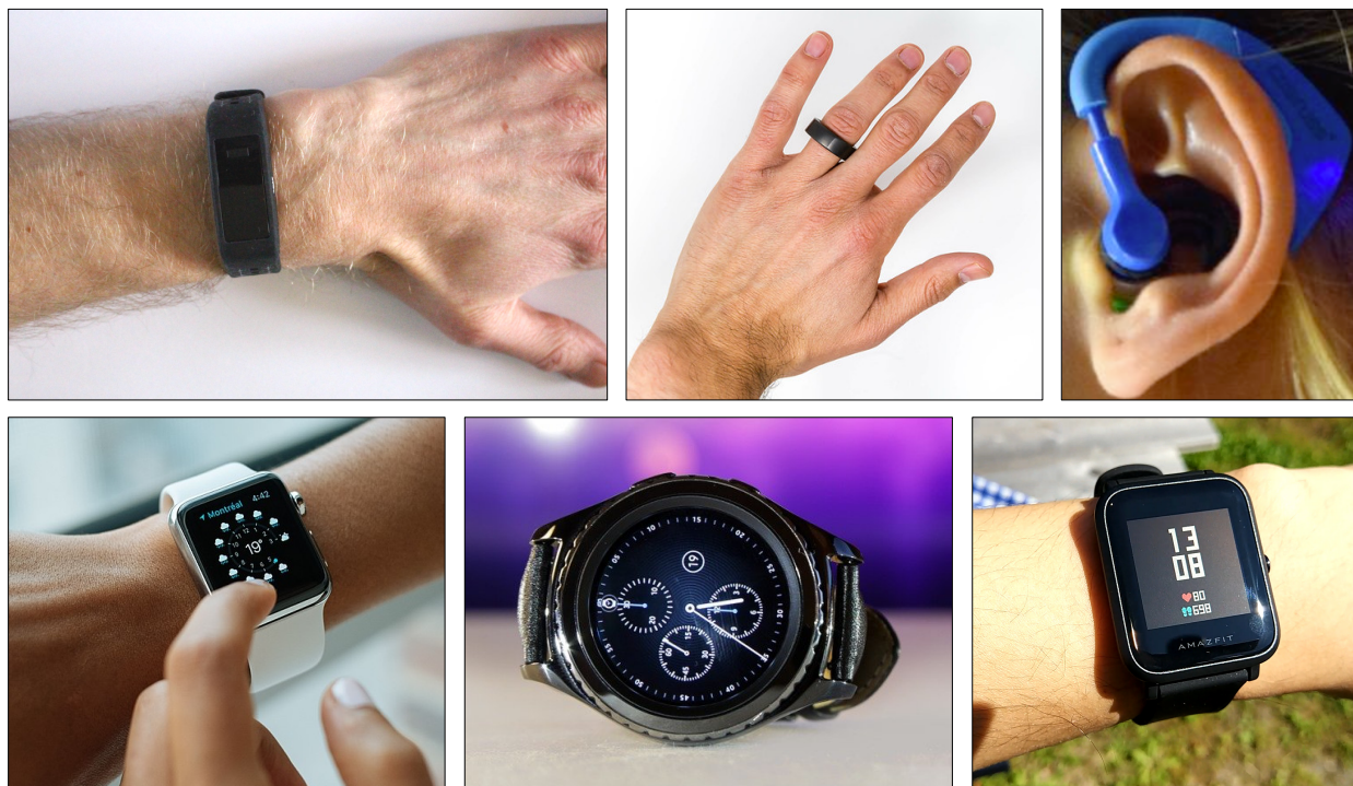
Fig. 7. PPG-based wearable devices: Examples of wrist-worn devices which measure the PPG signal. (clockwise from top left) The Max-Health-Band, Oura Ring, Amazfit Bip, Samsung Gear Galaxy S2, and Apple Watch.
