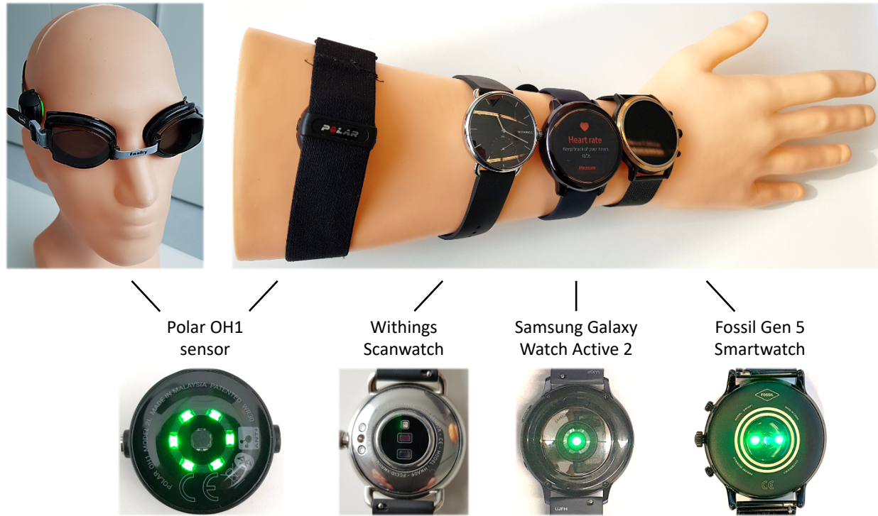
Fig. 3. Wearable photoplethysmography devices: Examples of wearables which measure the photoplethysmogram (PPG) signal, shown from above and the sensor side (below).
